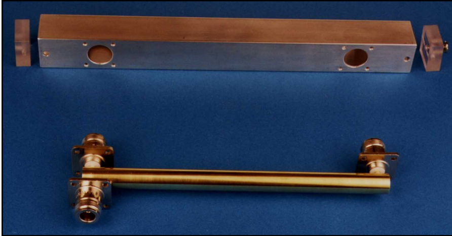
Fig 4—The parts ready for assembly. Do not solder the connectors to the center conductor before assembly! Secure one connector at each end to the square tube. Then fit and solder the center conductor to the center pins of the mounted connectors. Install the remaining connector and solder its center pin to the center conductor. Press the Lexan end plates in position and secure them with #4-40 machine screws.
